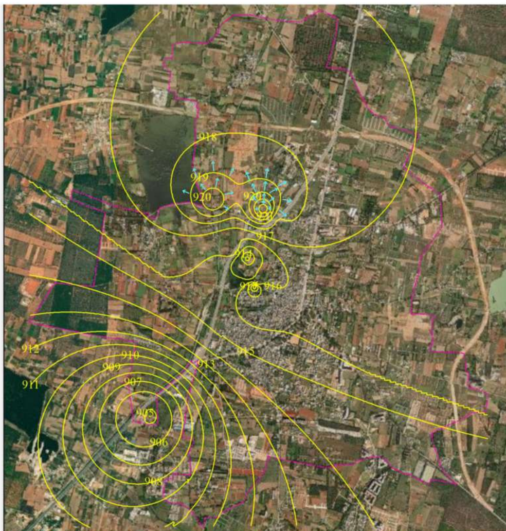
Image: water table contour map created using water level depth data obtained from 15 wells in the Devanahalli TMC.
